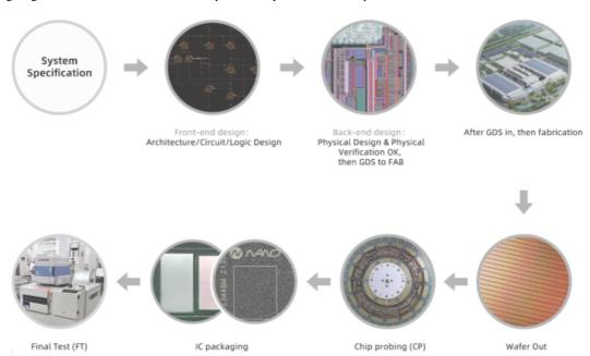
We design our IC products in-house. We determine the parameters of the IC products, establish the basic logic of the design, map out the initial plan for the physical layout, and conduct back-end verification on the
