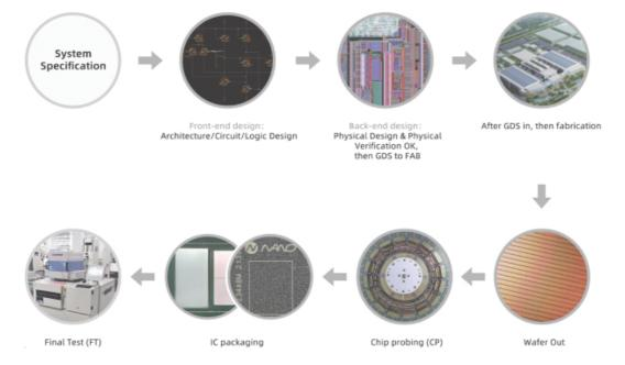
We design our IC products in-house. We determine the parameters of the IC products, establish the basic logic of the design, map out the initial plan for the physical layout, and conduct back-end verification on the
